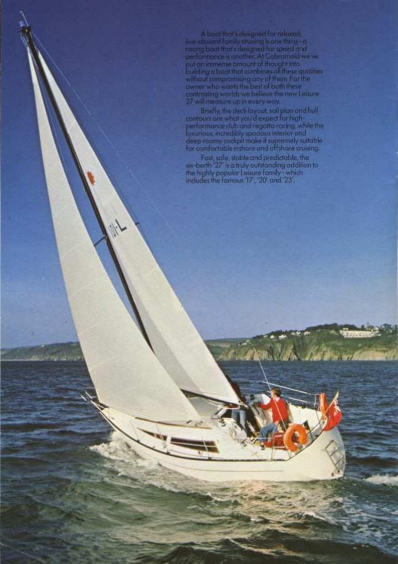
With the hull in solid GRP with foam ribs and stringers for exceptional strength and minimum maintenance, and deck in balsa sandwich for maximum insulation properties, the Frank Pryor designed '27' is 22' on the water line and has a generous 9'21/2" beam.
